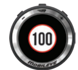
Speed Limit Indicator & Traffic Sign Recognition
